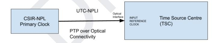
In case of CISR-NPL Primary Clock Site and TSC are collocated then the input reference to Time Source Centre will be provided by optical connectivity at optical interface. PTP will be provisioned between this optical connection. 1G optical/Electrical interface is required at the PTP GM for input reference from CSIR-NPL
