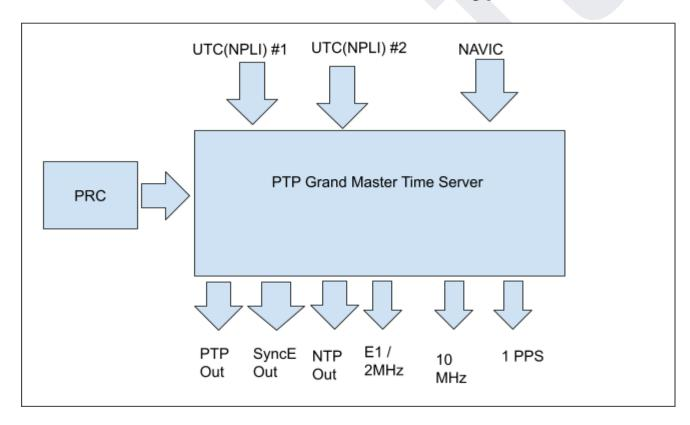
iii. TSC Type A would have an additional input source of PRC as per the GR (TEC 49170:2020) in comparison to Type B TSC. PRC will provide the hold over mechanism in case input references fail or become unavailable or spurious.
